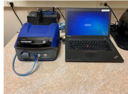
Fig. 8. Portacount® quantitative fit test device.
