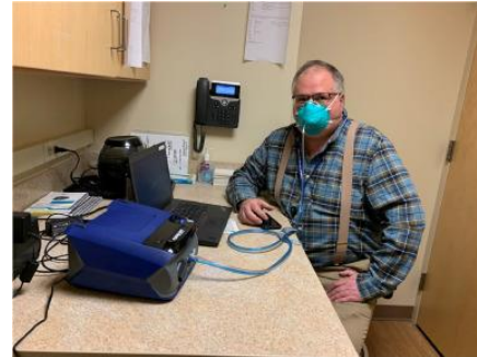
Fig. 7. Fit testing N95 mask with PortaCount®.
